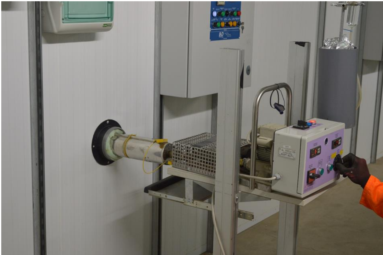
Figure 2. CEDAX Electrofog EWH-3000 for application of spearmint oil
