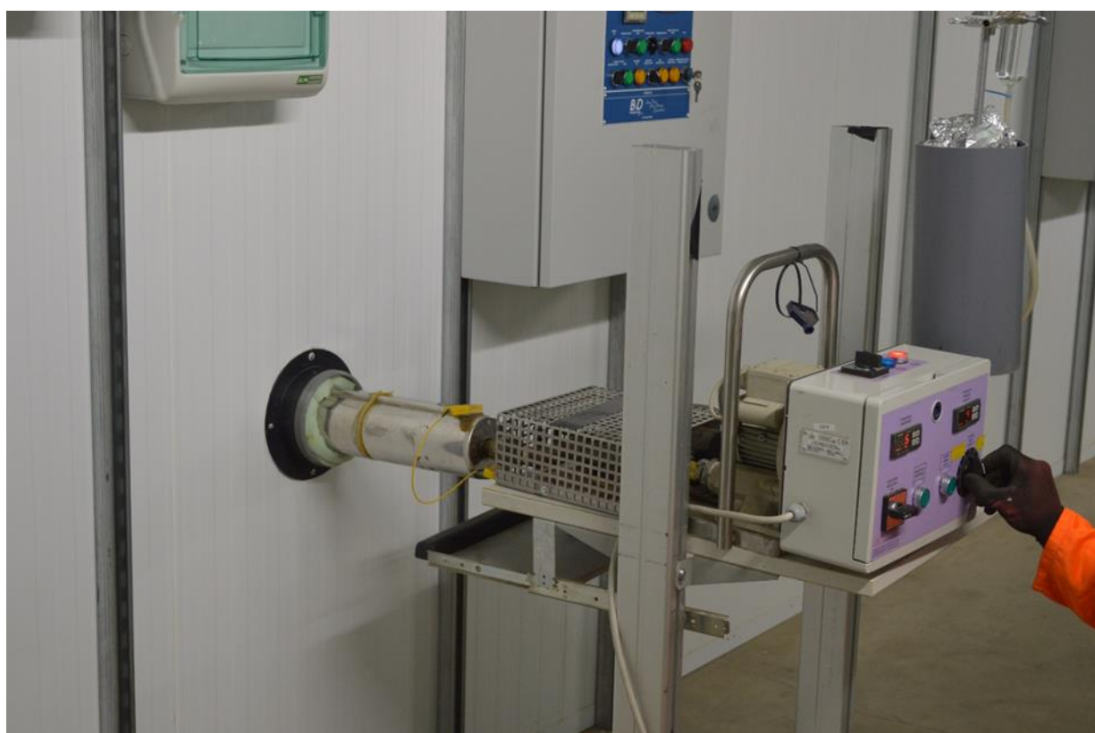
Figure 1. CEDAX Electrofog EWH-3000 used for application of DMN.
