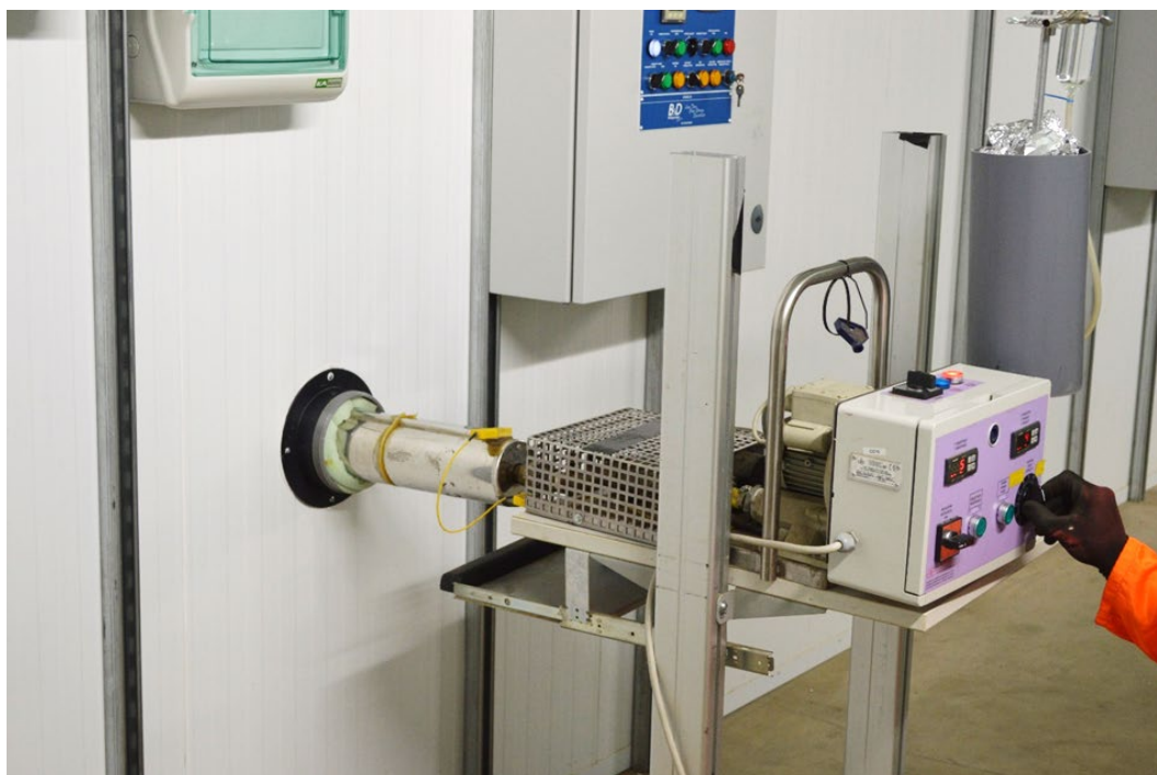
Fig. 2. CEDAX Electrofog EWH-3000 for application of spearmint oil, DMN and SmartBlock.
