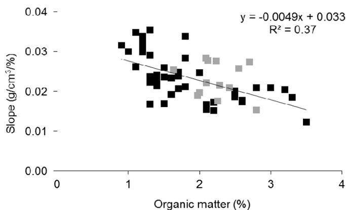
FIGURE 6. RELATIONSHIP BETWEEN THE SLOPE OF BULK DENSITY VS SOIL WATER CONTENT RELATIONSHIP AND THE MEAN ORGANIC MATTER PERCENTAGE IN EACH FIELD, 2009-2011. ■ 2011 DATA. SLOPE OF THE RELATIONSHIP:  $Y = -0.0049X + 0.033$ , PERCENTAGE VARIANCE ACCOUNTED FOR = 37 %.
