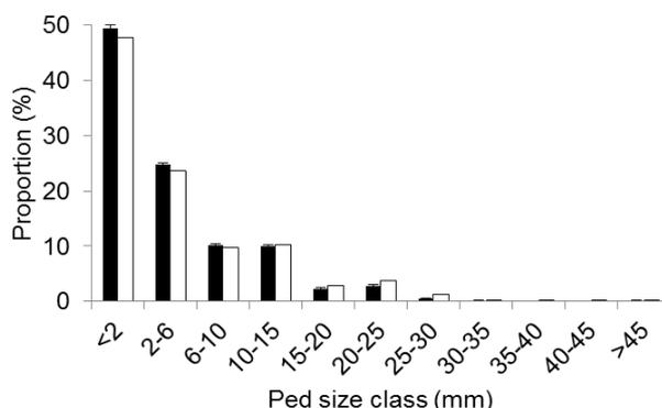
FIGURE 4. PED SIZE DISTRIBUTION IN EXPT 2. ■, NARROW STAR SPACING; □, WIDE STAR SPACING. DATA ARE MEANS OF TWO DESTONING DEPTHS.
