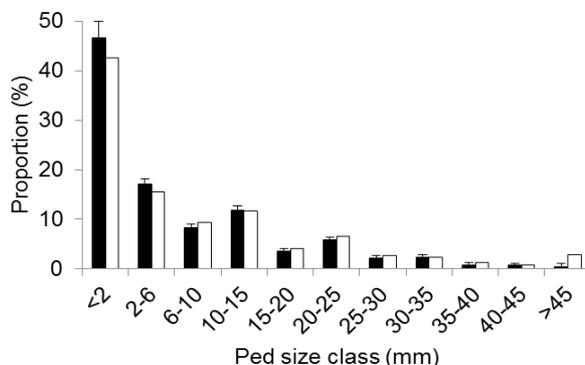
FIGURE 3. PED SIZE DISTRIBUTION IN EXPT 1. ■, SHALLOW DESTONING; □, DEEP DESTONING. DATA ARE MEANS OF TWO N LEVELS.
