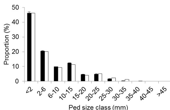
FIGURE 5. PED SIZE DISTRIBUTION IN EXPT 3. DATA ARE MEANS OF TWO HOOD PRESSURES AND THREE HOOD TYPES. ■, SHALLOW DESTONING; □, DEEP DESTONING.
