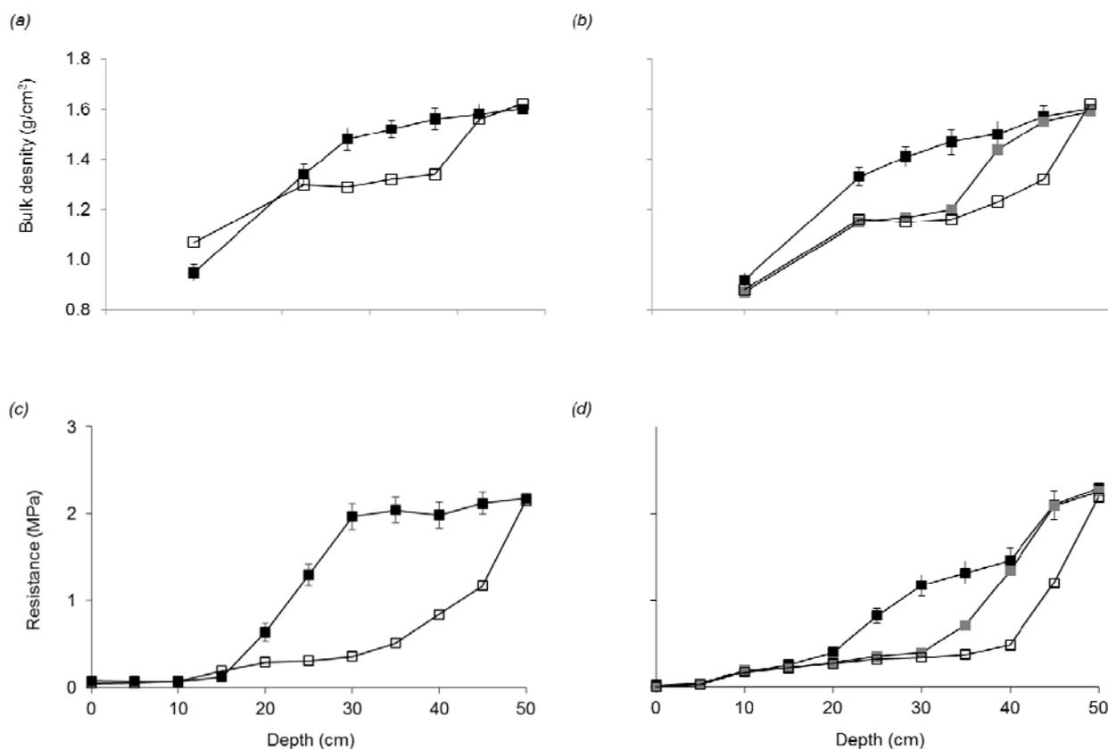
FIGURE 2. EFFECT OF DESTONING DEPTH ON SOIL BULK DENSITY AND PENETRATION RESISTANCE. BULK DENSITY: (A) EXPT 1; (B) EXPT 2. RESISTANCE: (C) EXPT 1; (D) EXPT 2. ■, SHALLOW; ■, NORMAL; □, DEEP. MEAN OF TWO N REGIMES IN EXPT 1 AND TWO AGGRESSIVENESS TREATMENTS IN EXPT 2.
