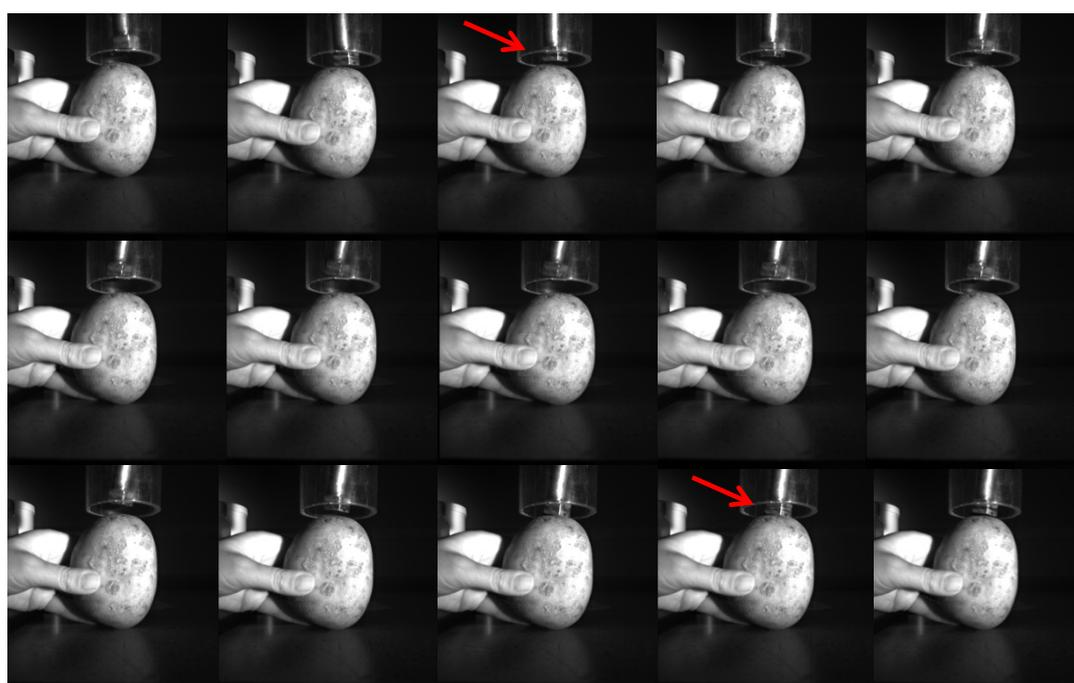
Figure 4.4. Impact on the stolon end of the potato using falling bolt. Images from high speed camera every 0.02 sec. Arrows indicate contact between bolt and tuber.
