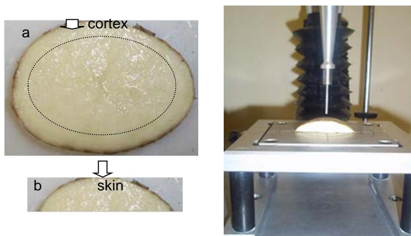
Figure 3.2 Transverse section with the points analysed with penetration test. a, cortex; b, skin cortical layer.
