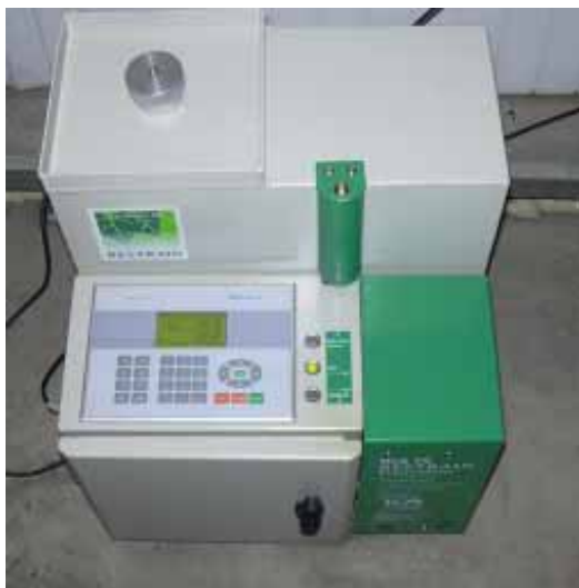
FIG. 3. RESTRAIN ETHYLENE CONTROL SYSTEM. ETHYLENE IS GENERATED CATALYTICALLY USING ETHANOL FROM AN INTEGRAL STORAGE TANK.
