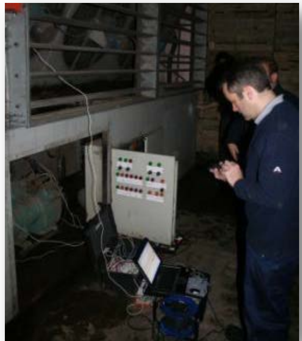
Figure 3.6.6 - Compressor wired for ClimaCheck monitoring
