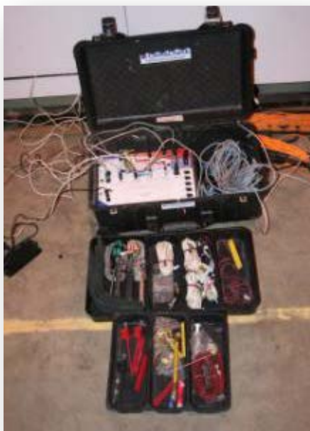
Figure 3.6.2 - ClimaCheck monitoring system
