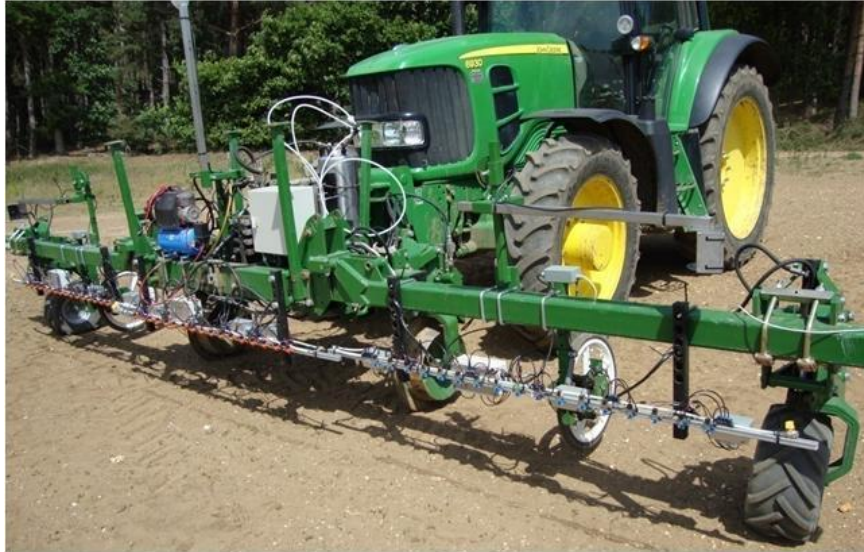
Figure 23. The experimental rig as set up for the field trials in the onion crop in the 2011 cropping season. Note the new nozzle/valve assembly design (in orange) fitted to the two booms on the far side of the machine and nozzle/valve assemblies from the previous project (in blue) fitted to the nearside boom.
