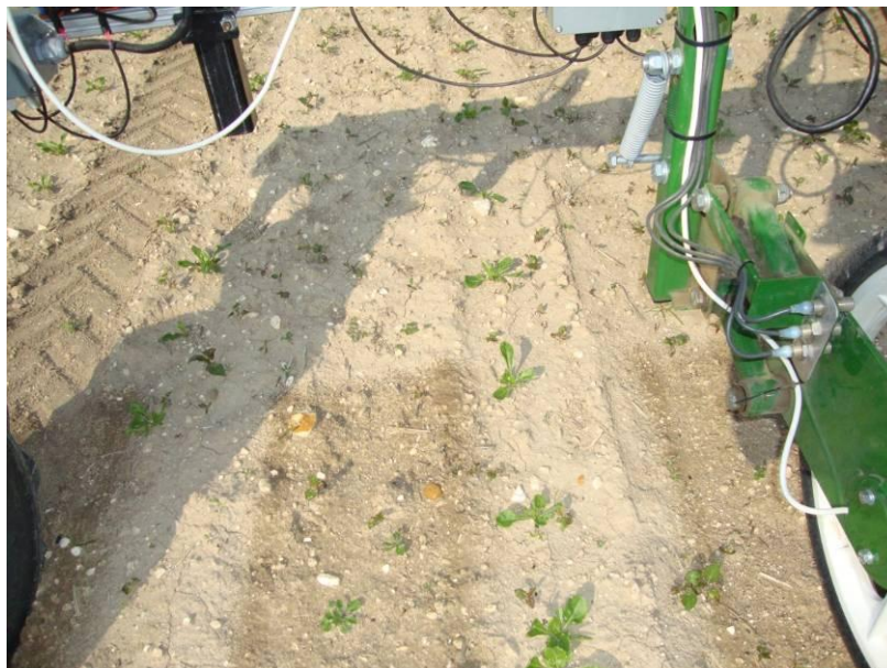
Figure 43. Crop and weed conditions for the sugar beet experiments in May 2012. Main picture – field condition showing unsprayed tramlines used for the experimental treatments on the right hand side of the picture. Inset – close up of crop and weed conditions.
