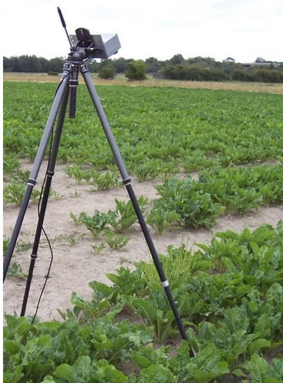
Figure 27. Stereo camera specially constructed to take stereo images of weed beet
