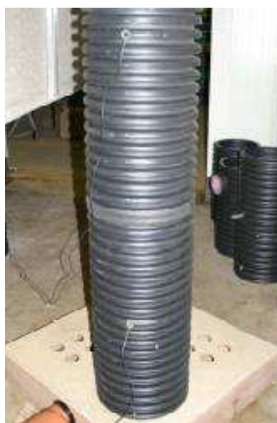
FIGURE 2. TWO METRE BY 0.3M ID PIPE CONTAINING C. 60 KG POTATOES. THE VAPOUR SOURCE WAS LOCATED ABOVE THE MANIFOLD, IN THE BOTTOM 50CM SECTION OF PIPE.
