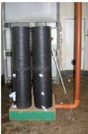
FIGURE 16. LAYOUT OF PLENUM WITH THREE PIPES CONTAINING SAMPLES AND SUPPLIED WITH CLEAN AIR, AS USED IN CIPC REDISTRIBUTION TRIAL.
