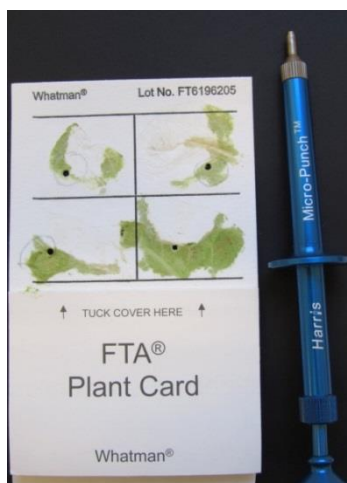
Figure 3. An example of an FTA card showing the micro-punch and the location of the disks cut from each lesion imprint.
