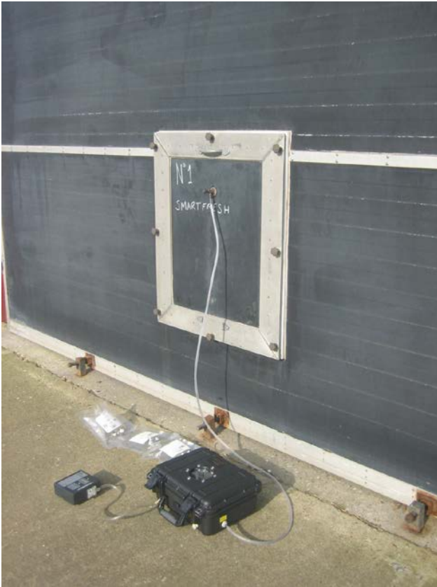
Figure 3: Sampling of the store atmosphere during the storage period, using Teflon air sampling bags and a vacuu-chamber.
