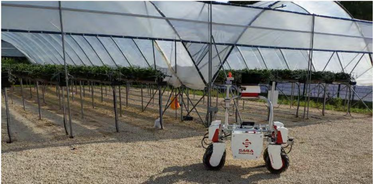
Figure 1: Thorvald robot adjacent to strawberry tabletop plantation at the University of Lincoln Riseholme campus. This Thorvald is equipped with 3 realsense cameras; RGB, depth, one Raspberry Pi Zero, one raspberry pi camera v2, one BME680; temperature, humidity, and air- quality sensor
