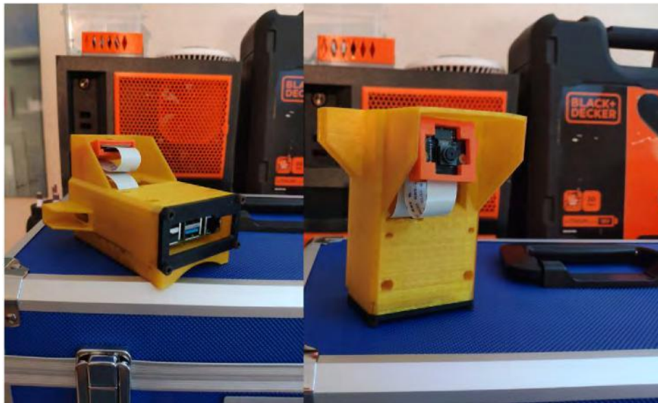
Figure 4: Raspberry pi stationary camera, used separately to the Thorvald robot, used to intensively monitor fewer strawberries over a longer period.
