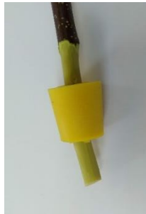
Figure 8 - Branch with phloem removed, inserted in a rubber bung for sap extraction. Photo taken on 18/03/2020
