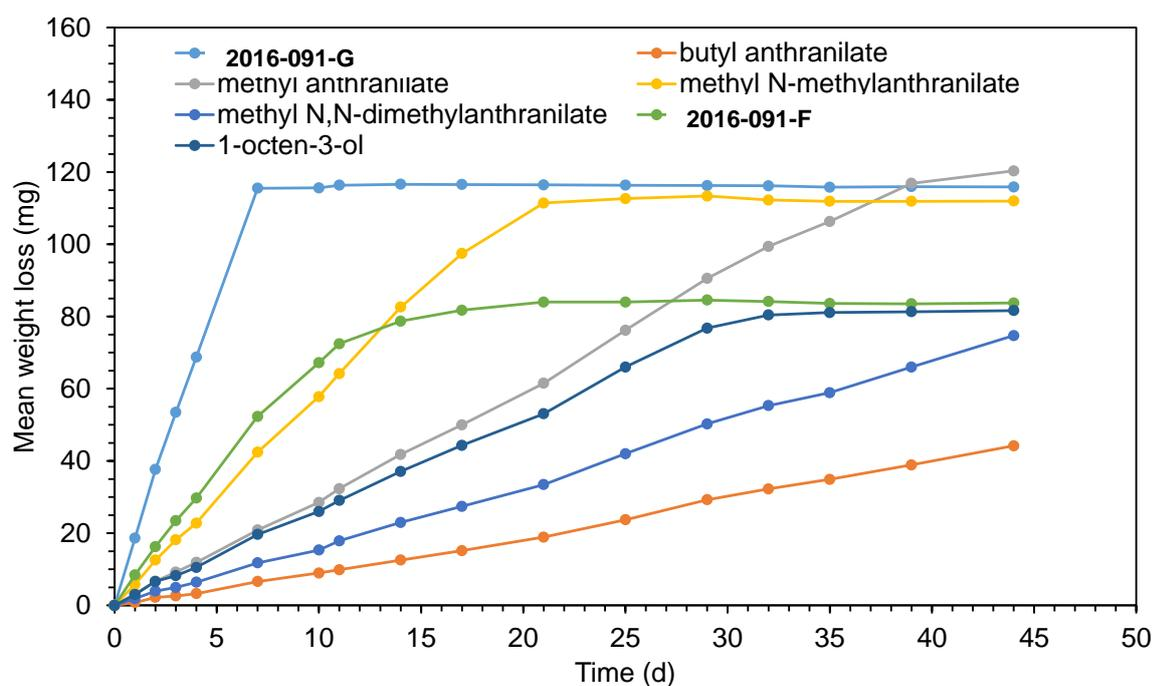
**Figure 5.2.1.** Release rates of candidate repellents (100  $\mu$ l) from sachets at 22  $^{\circ}$ C as measured by weight loss (sachets 5 cm x 5 cm x 120  $\mu$  thick; mean of two)
