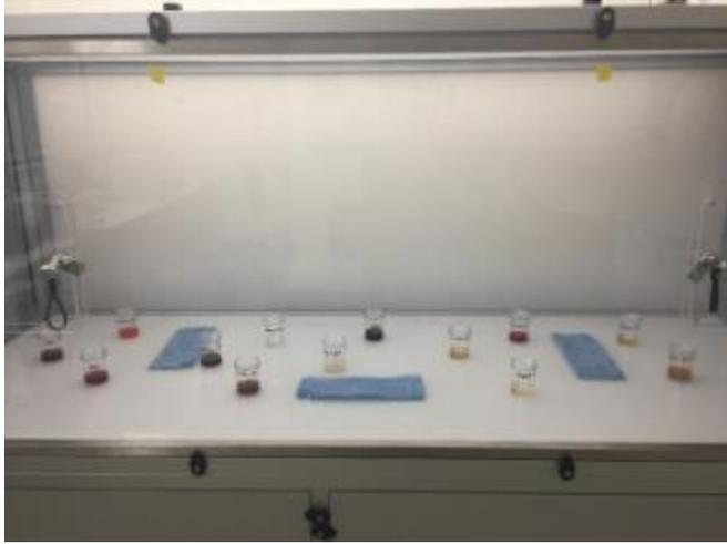
**Figure 5.1.1.** Large arena bait test showing positioning of open containers with test substances
