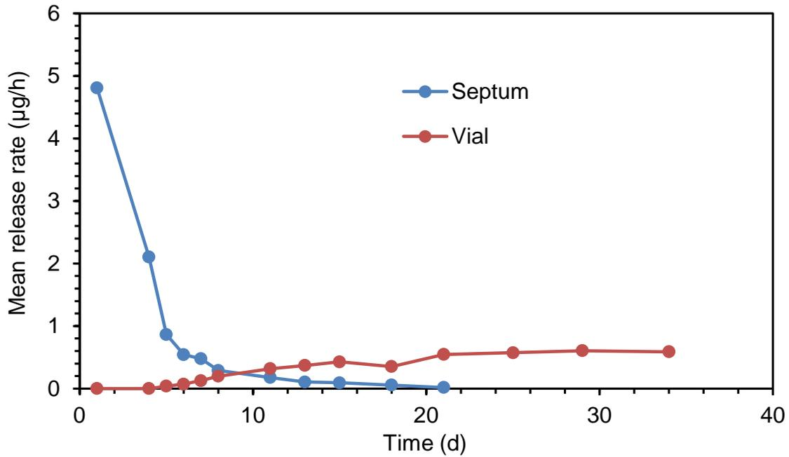
**Figure 5.2.2.** Release of geosmin (4 mg) from rubber septa or polyethylene vials at 27 °C as measured by collection of volatiles (mean of two replicates)
