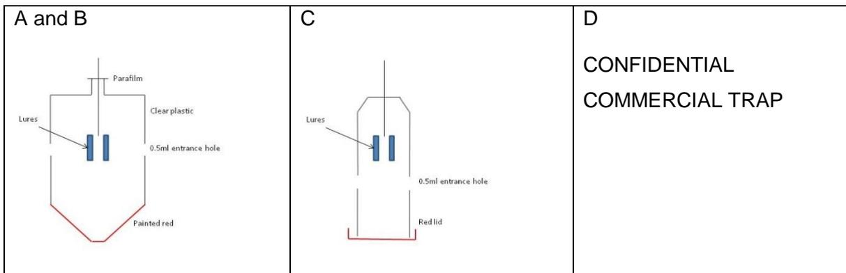
**Figure 4.2.7.** Devices used A and B) 175 ml Falcon tube, C) 50 ml Falcon tube, D) Commercial dry trap (Coded)
