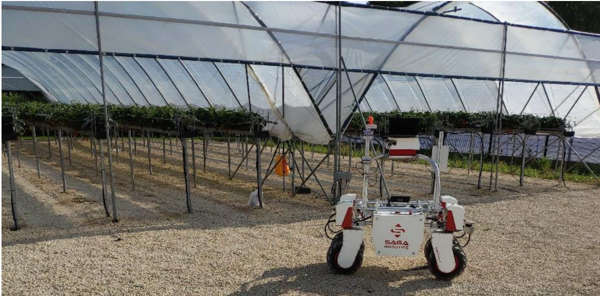
Figure 2: Thorvald robot adjacent to strawberry tabletop plantation at the University of Lincoln Riseholme campus. This Thorvald is equipped with 3 realsense cameras; RGB, depth, one Raspberry Pi Zero, one raspberry pi camera v2, one BME680; temperature, humidity, and air-quality sensor
