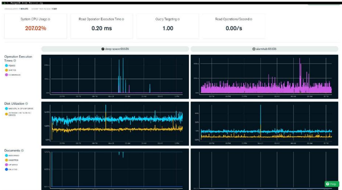
Figure 5: MongoDB, and monitoring. This allows us to continuously be aware of the state of the replica sets, their load, who is the master/ primary, network traffic, etc. This is an invaluable resource to the management of such a system and will provide us with many useful tools to analyze the effects of our research on this distributed implementation.
