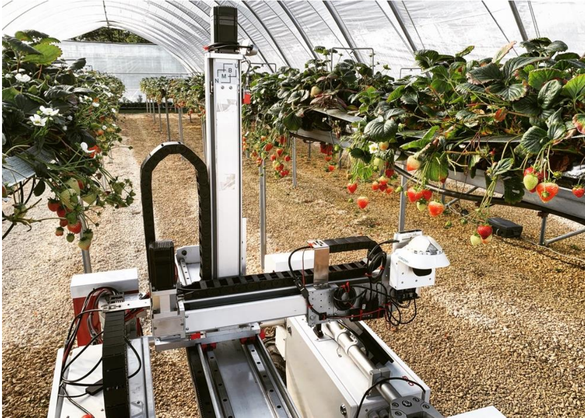
Figure 4: Strawberry harvester mounted on the Thorvald platform harvesting berries using the object detection approaches mentioned above.
