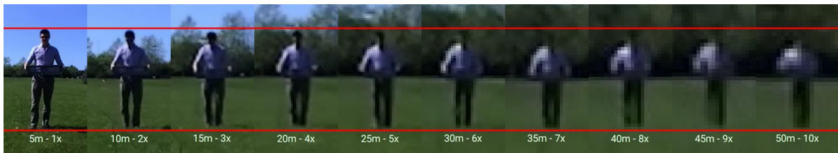
Figure 5. An indication of resolution of a human at increasing distance from the camera, highlighting the human detection problem over longer distances.
