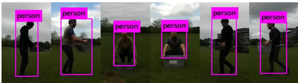
Figure 6. Examples of person detection whilst performing actions with crates, using the YOLOv3 algorithm.
