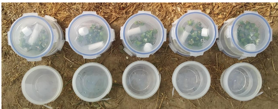
Figure 2.2. Top row: five replicate extraction devices, each containing 20 button fruits and an open MIK dispenser in the top chamber. Bottom row: five corresponding pots of 70% ethanol for button fruits to be transferred to after MIK fumigation
