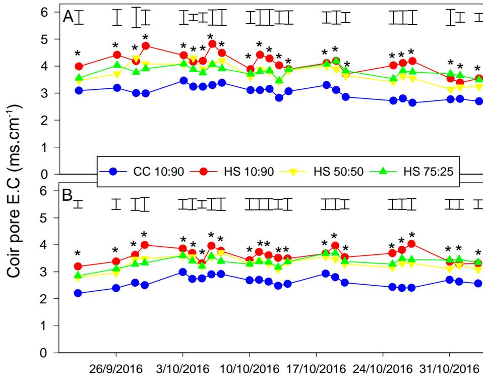
**Figure 2.** Average bag coir pore E.C. “Sonata” when measured A) directly underneath a plant and B) averaged from 3 positions (directly under a plant, directly under a dripper and mid-way between the two) from “spot” measurements made with a Delta-T “WET” sensor. Asterisks (\*) indicate significant differences between the treatments. Error bars represent LSD at 5%.
