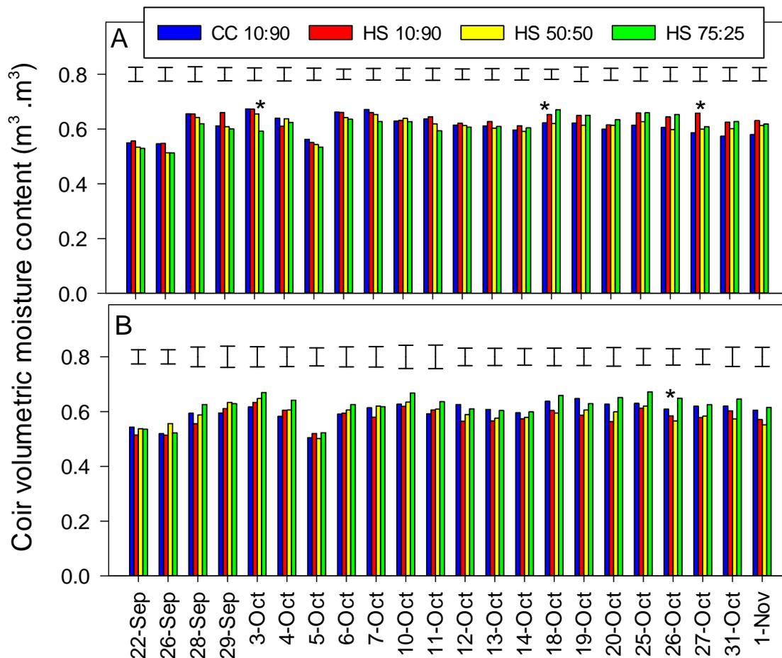
**Figure 1.** Average bag CVMC in A) “Sonata” and B) “Vibrant”, from “spot” measurements made with a Delta-T “WET” sensor, averaged across 3 positions within a bag, directly under a plant, directly under a dripper and mid-way between the two. Asterisks (\*) indicate significant differences between the treatments. Error bars represent LSD at 5%.
