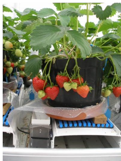
Figure 3. Decagon ECRN-50 rain gauges were used to measure volumes of run-off. Photo taken on 12 April 2016.
