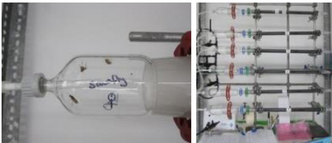
Figure 4. Sawfly females in collection chamber and equipment for collection of volatiles from gooseberry sawfly
