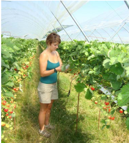
Figure 10. Spot measurements of soil volumetric moisture content, bulk EC and temperature were made weekly with a Delta-T 'WET' sensor. Photo taken on 26 July 2012.
