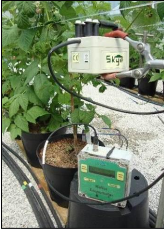
Figure 5. The Skye Evapo-sensor and Evapometer used to estimate daily potential evapotranspiration. Photo taken on 15 July 2010.
