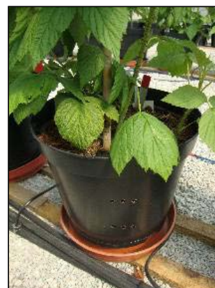
Figure 5. Insertion points for the WET sensor probe on the N side of the pot. Photo taken on 9 July 2010
