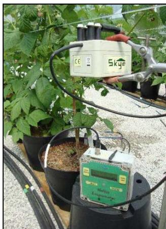
**Figure 4.** The Skye Evapo-sensor and Evapometer used to estimate daily potential evapotranspiration. Photo taken on 15 July 2010
