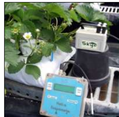
Figure 4. The Skye Evaposensor and Evapometer used to estimate potential evapotranspiration. Photo taken on 4 August 2009
