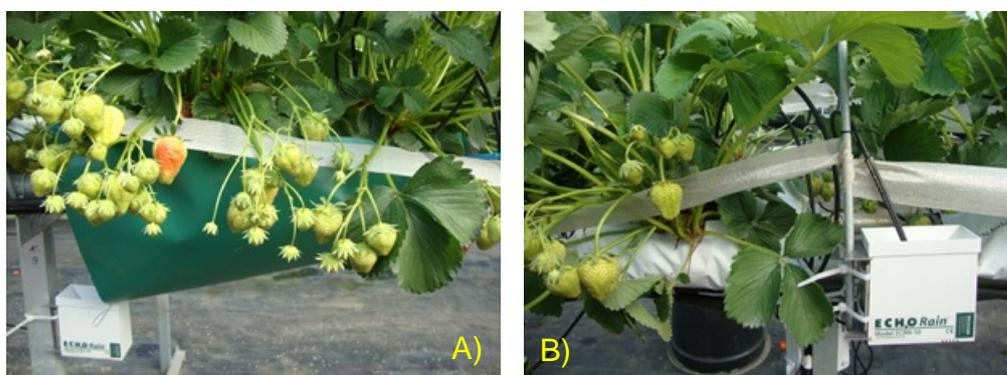
**Figure 4.** Rain gauges were used to record A) volumes of run-off and B) dripper outputs automatically throughout the season. Photos taken on 9 May 2011, the experiment shown was carried out as part of WU0110.
