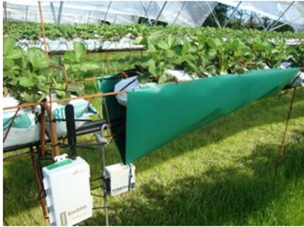
**Figure GS4.** Rain gauges and data loggers with telemetry are being used to record water input and output volumes in grower trials in SF 136.
