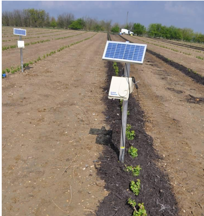
Figure 1. PAS 100 green waste mulched rows with Enviroskans™ – 13 April 2012 Coggeshall Hall Farm, Essex
