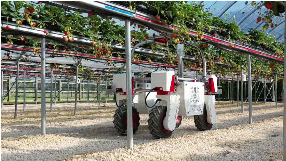
Figure 1.2: Sensors mounted on a robotic platform for data capture in polytunnels.
