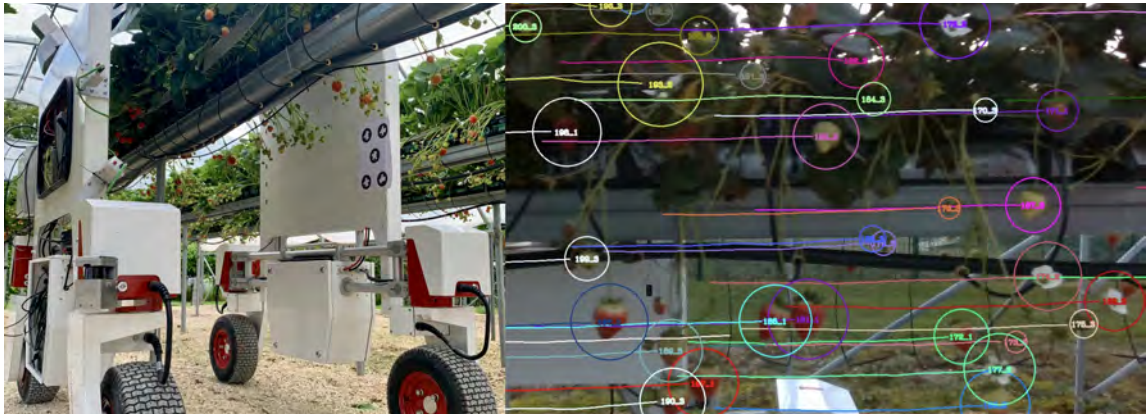
Figure 5.1: Mobile robot tracking platform in the Katrina-1 Strawberry row (left). Fruit counting-by-tracking (Ripe, Unripe and Flower) visualisation (right). The circles show the tracked fruit identities over time and tracks generated from our proposed method. Strawberry maturity classes are omitted for visualisation purposes, individual instances are in the format TrackID_ClassID where 1, 2, 3 are ripe, flower and unripe respectively.
