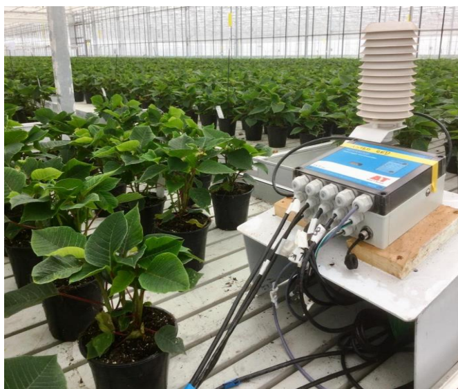
Figure 3. The GP2 Advanced Datalogger and Controller on the bench in the “Astro Red” irrigation block. The SM150T sensors are hard-wired into the ports into the datalogger. Source; Else, 2018
