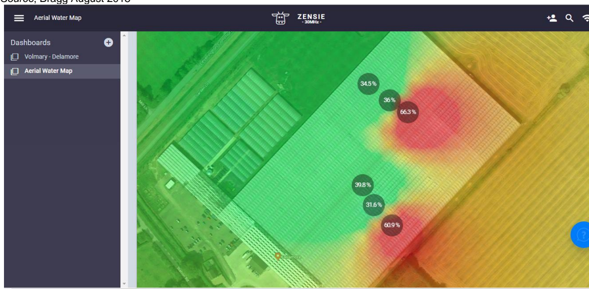
Figure 10. Ariel view of water map from wireless sensor data at Volmary nursery, red indicates wetter areas. Source; Bragg August 2018
