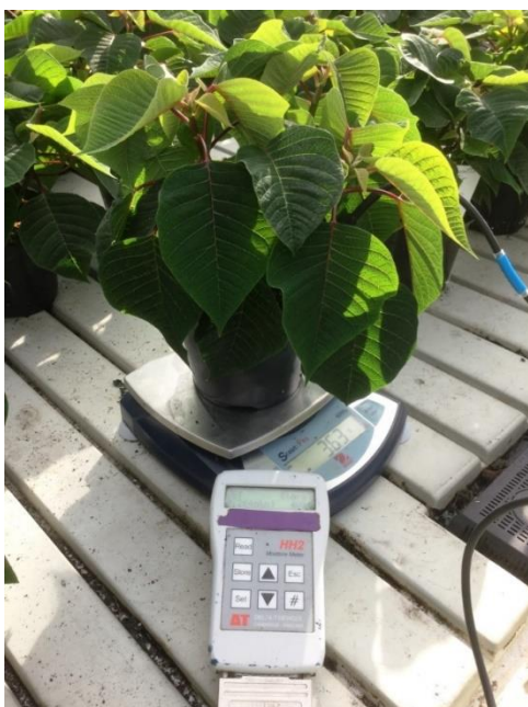
Figure 6. Plant-and-pot weights were measured with an electronic balance and spot measurements of SVMC were made with a Delta-T “WET” sensor. Source; Else, 2018
