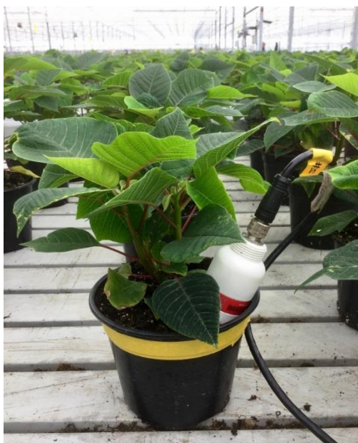
Figure 4. An SM150T sensor buried into the substrate to record changes in SVMC in an “Astro Red” plant. Source; Else, 2018
