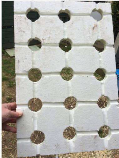
Figure 9. Modified air gap by the addition of channels to produce uninterrupted air flow.
