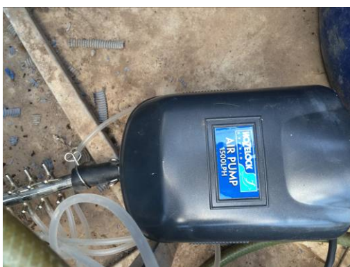
Figure 17. Air pump to increase oxygen levels in the pool.
