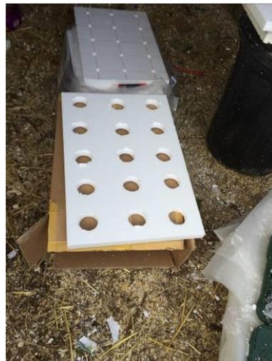
**Figure 4.** A completed float of 50 mm air gaps.
