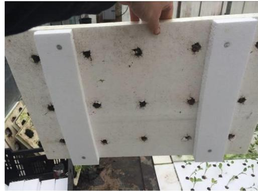
**Figure 10.** Air gap created by the use of thin strips of polystyrene.
