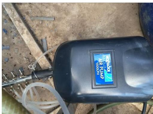
**Figure 17.** Air pump to increase oxygen levels in the pool.
