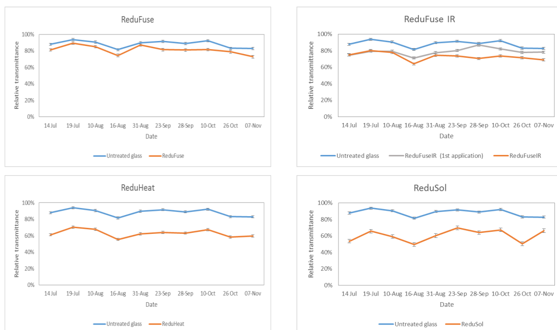
Figure 19. Mardenkro products: relative light transmission. The data presented is the light transmission data for treated (brown line) and untreated (blue line) glass expressed as a percentage of sunlight; data was recorded simultaneously under the product and as direct sunlight. Data points are an average of three measurements taken either beneath the treatment or under direct sunlight, which were then averaged across the three replications (i.e. from three panes of glass). The grey line represents data recorded from the first application (AP1); this data is an average of three measurements taken either beneath the treatment or under direct sunlight, but was not replicated (i.e. from one pane of glass)
