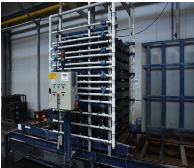
Figure 20. Fertigation rig for tulip bulbs in crates
