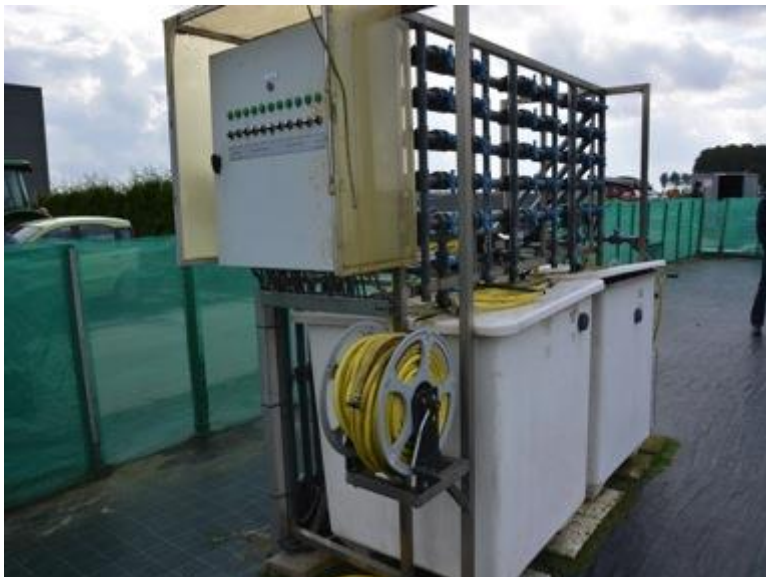
Figure 28. Irrigation control rig for solution hydroponics
