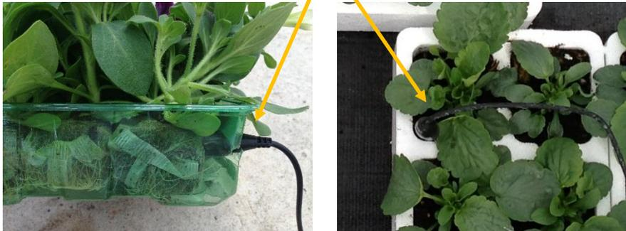
**Figure 3.** Positioning of SM100 Soil Moisture Sensor within a coir system, inserted horizontally (image left); and in a peat based system inserted vertically (image right) production systems
