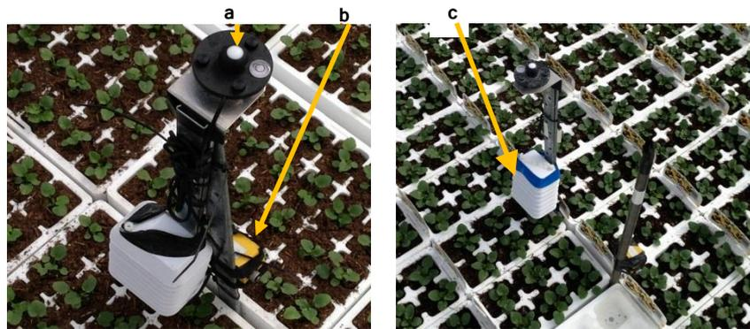
**Figure 2.** Positioning of data loggers and light sensor within a batch of pansies: a) LightScout Quantum Light 3 Sensor PAR probe; b) Tinytag Plus 2 data logger (temperature and humidity); c) Watchdog 1000 series data logger housed within a radiation shield for protection against solar radiation and water damage
