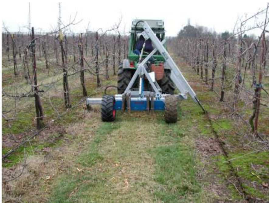
Figure 1. Root pruning during the dormant season in Cox. Note the use of an angled blade on the right hand side of the picture in the treated rows and a vertical blade on the left hand side of the picture in the guard row.
