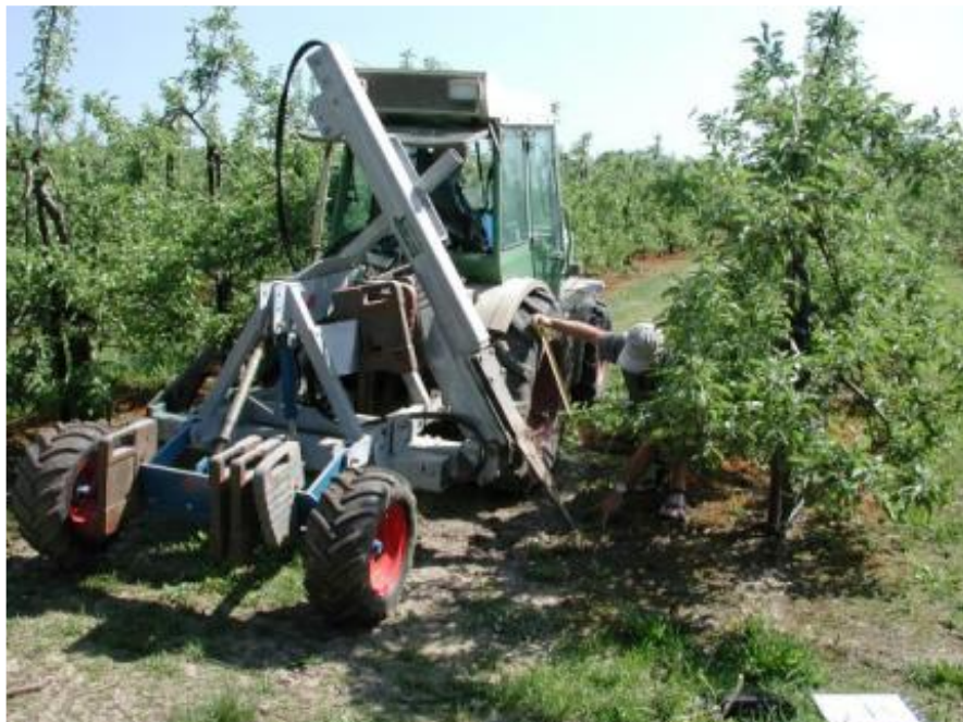
Figure 3. Setting the blade of the root pruner to 90 cm from the tree in Cox.
