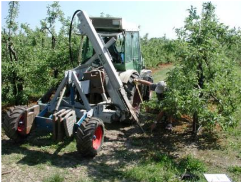
Figure 5. Setting the blade of the root pruner to 90 cm from the tree on Cox.
