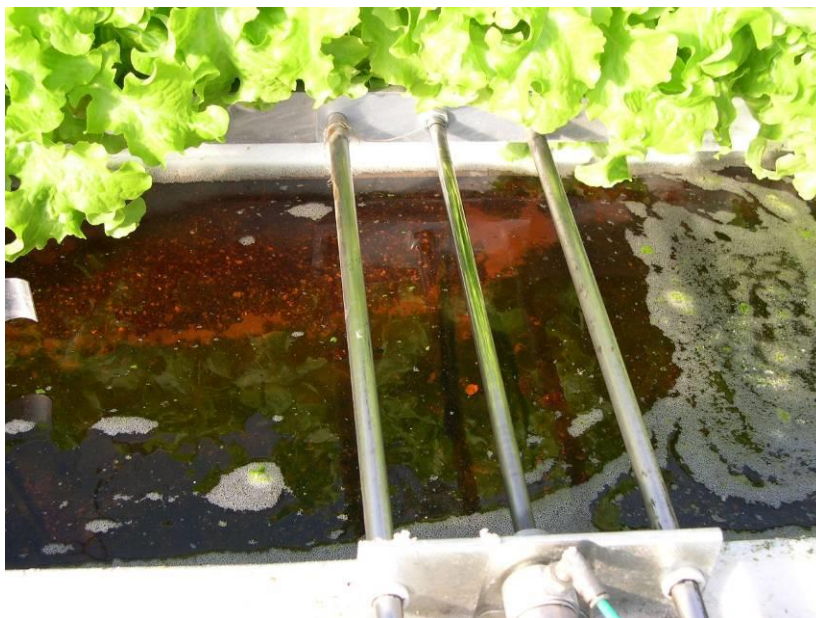
Plate 8: Close-up of the automated push rod mechanism for moving the polystyrene rafts around the platforms
