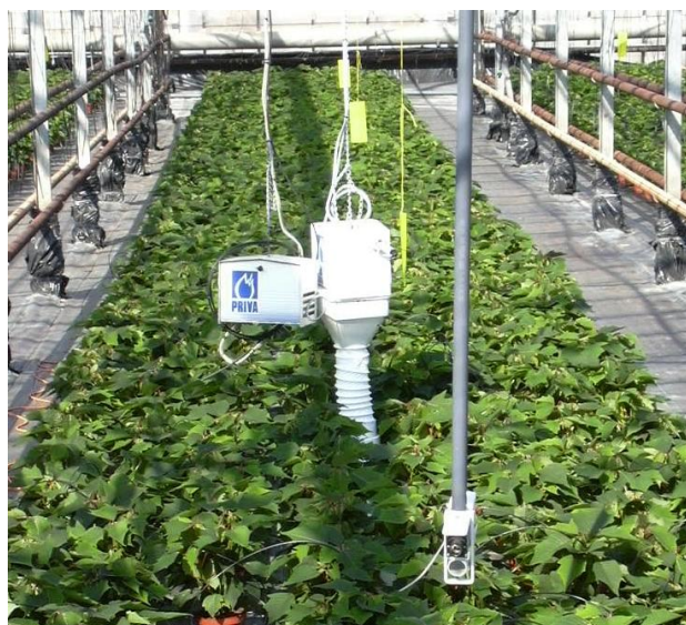
Fig 5 – Normal next to Canopy with infra-red camera in foreground
