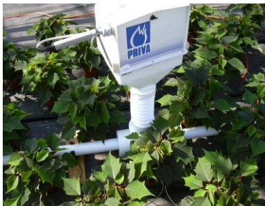
Figure 1: Canopy measuring box
