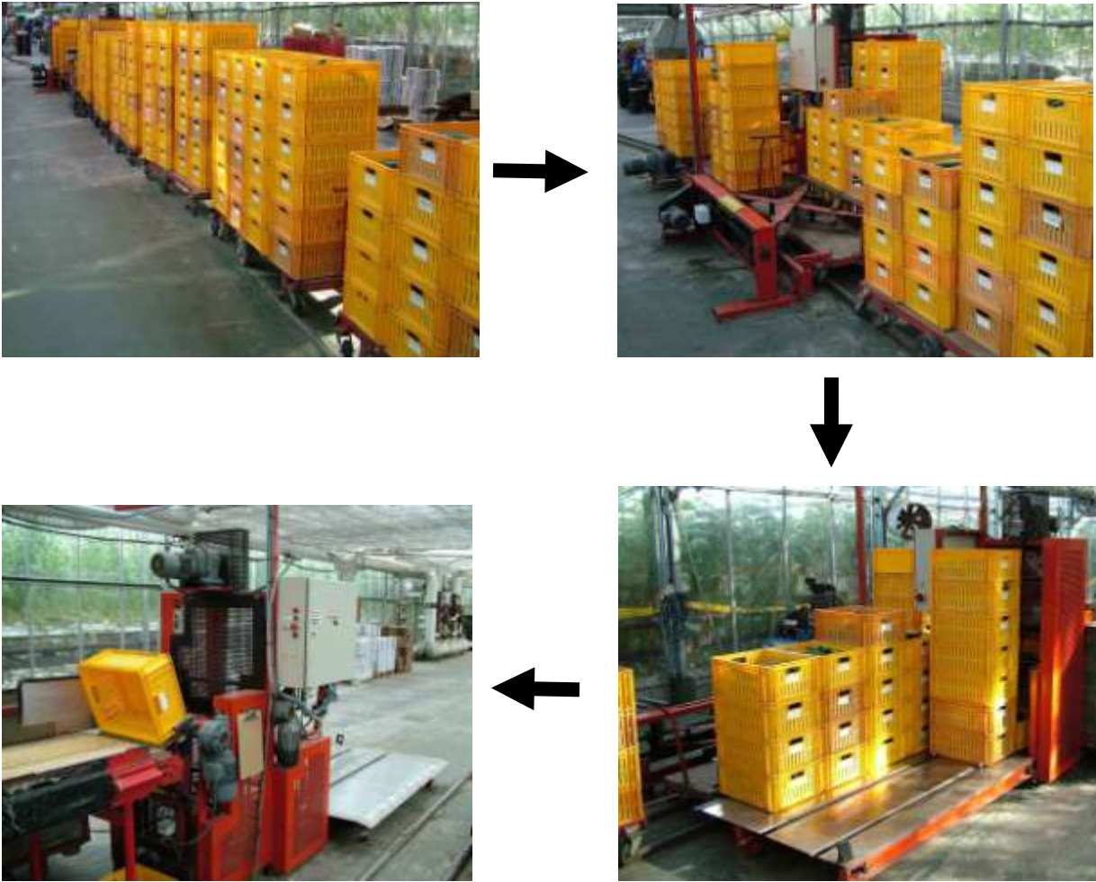
Figure 1.14: Picking cart transport with automatic de-stacking and tipping
