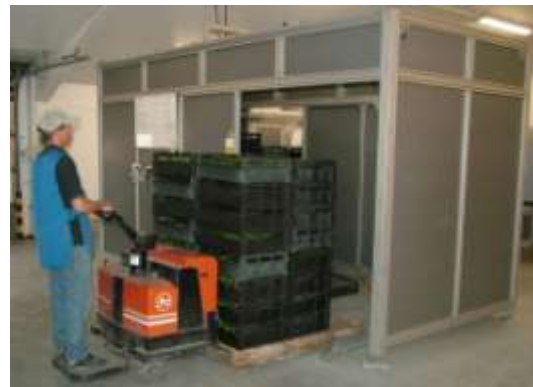
Figure 1.13: Palletised boxes with automatic de-stacking and tipping
