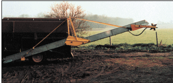
Figure 3 – The mixer loader system
