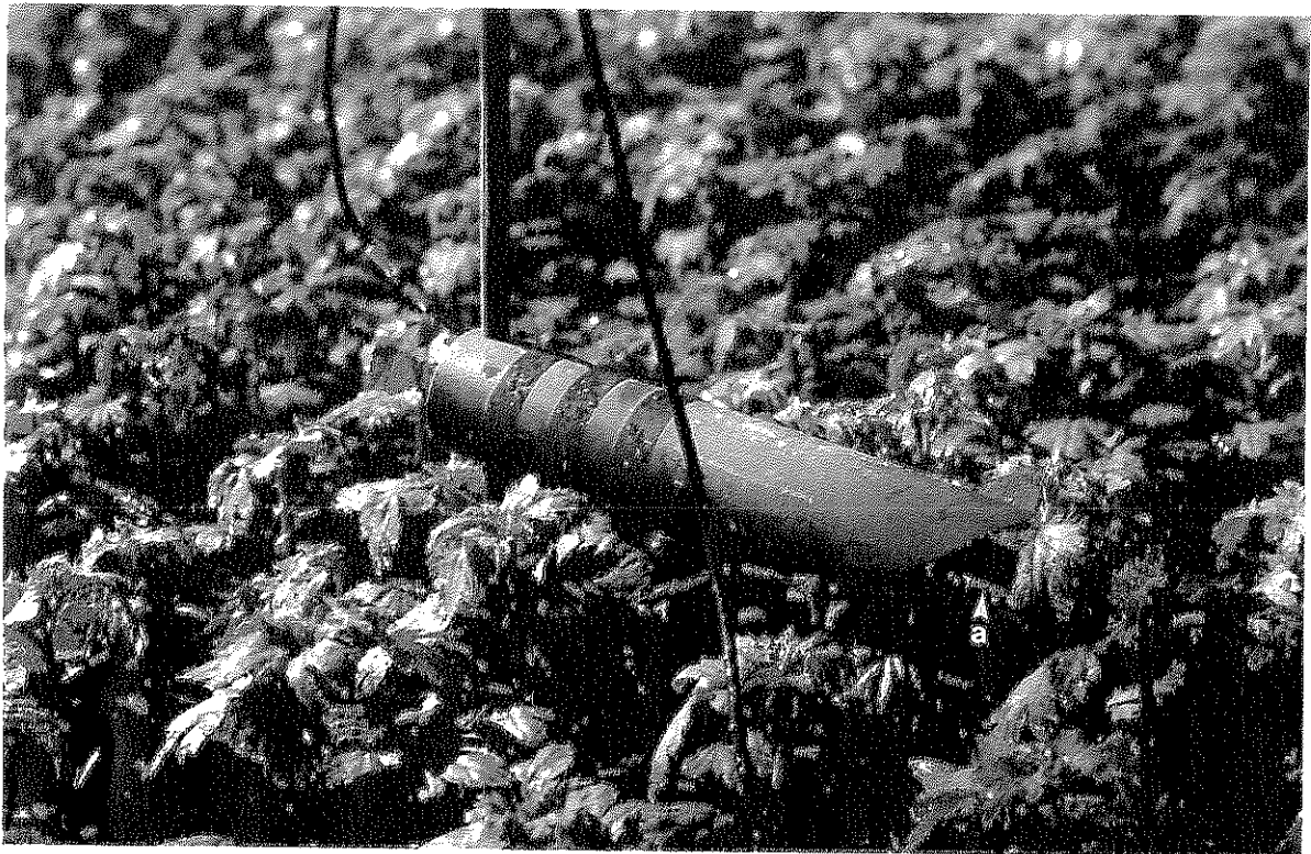
Plate 2 : Humidity probe (a) and leaf thermistor (b) for measuring canopy microclimate
