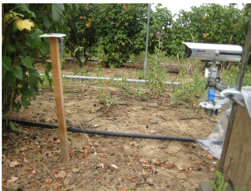
Figure 3.D.1. Photograph of camera and lure set up in field to record male L. pabulinus behaviour
