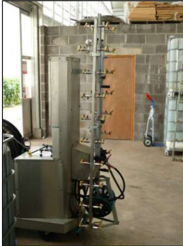
Figure ii. New booms fitted to the robotic sprayer:
