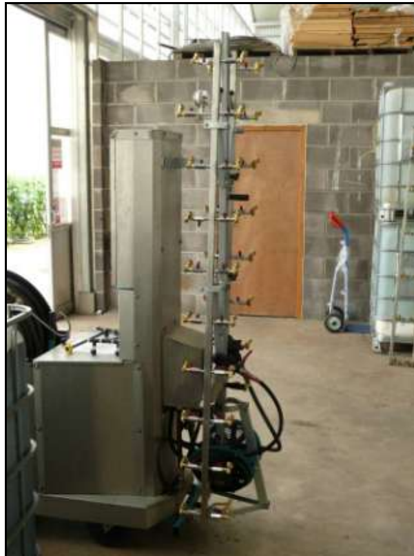
Figure 4. New booms fitted to the robotic sprayer
