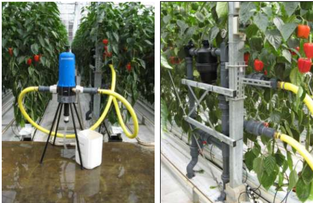
Figure 15. Dosatron in situ showing stock tank (white container) and connections to manifold
