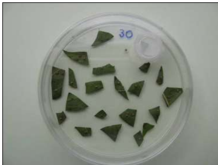
Figure 10. Ventilated incubation dish as used for parasitoid emergence tests
