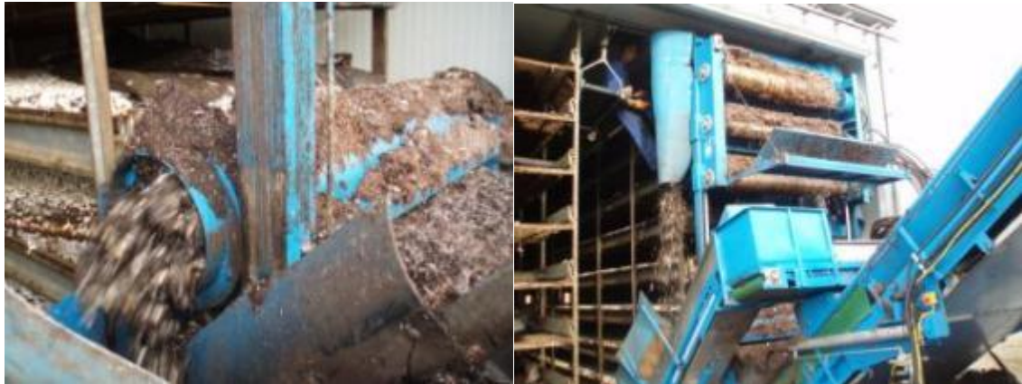
Fig. 1. MushComb casing separator in use at a shelf farm in the Netherlands
