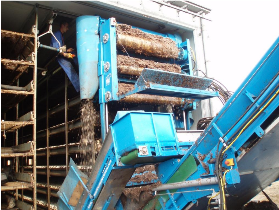
Fig. 1. MushComb casing separator in use at a shelf farm in the Netherlands
