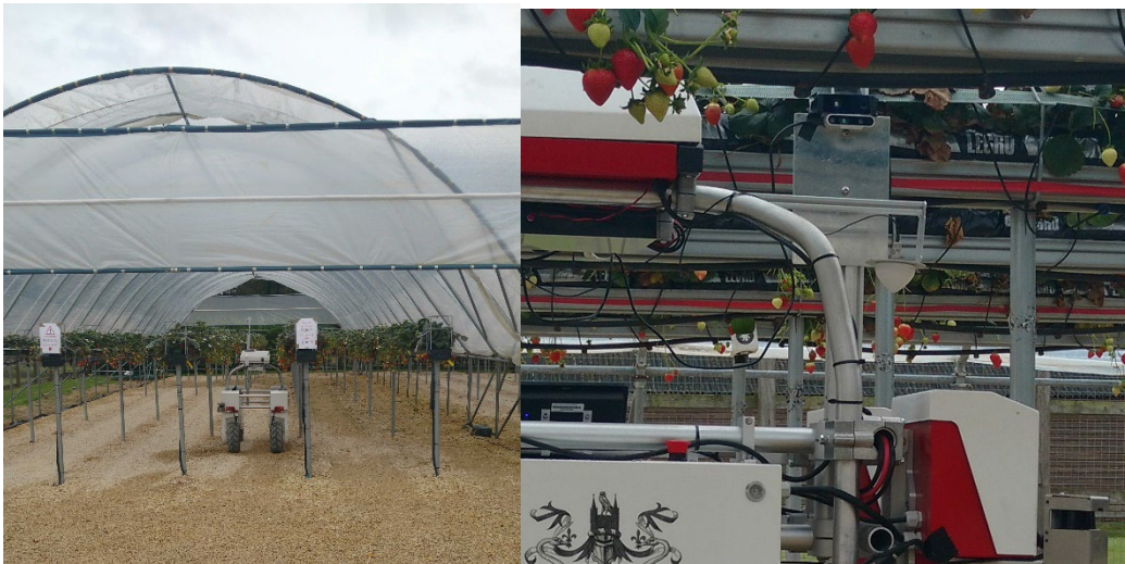
Figure 1: The Thorvald robot in the strawberry polytunnels, with camera mounted for fruit analysis.
