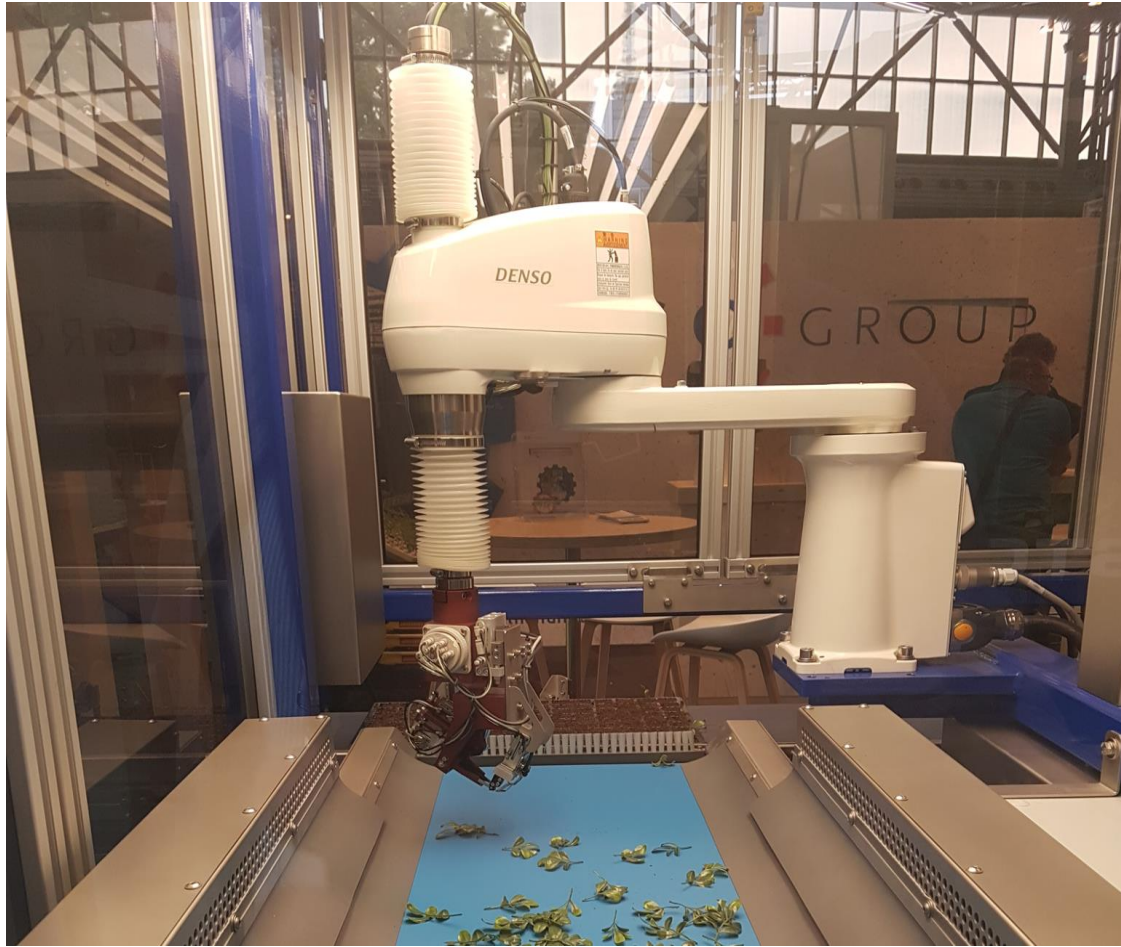
Figure 1: Precision agriculture system used for planting cuttings (foreground) into standard plant trays (background). Uses a SCARA robot for high-speed pick and place with a custom gripper and vision system.
